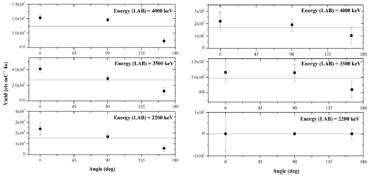
**Fig. 3:** Angular distributions of the  $\gamma$  rays of the reaction  $^{107}\text{Ag}(p,\gamma)^{108}\text{Cd}$  (left) and  $^{109}\text{Ag}(p,\gamma)^{110}\text{Cd}$  (right). The distribution pattern was assumed to be flat.
