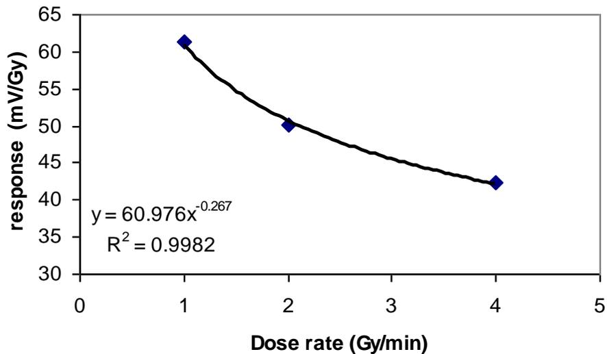
**Figure 3.** The dose response as a function of the dose rate of the electron irradiation
