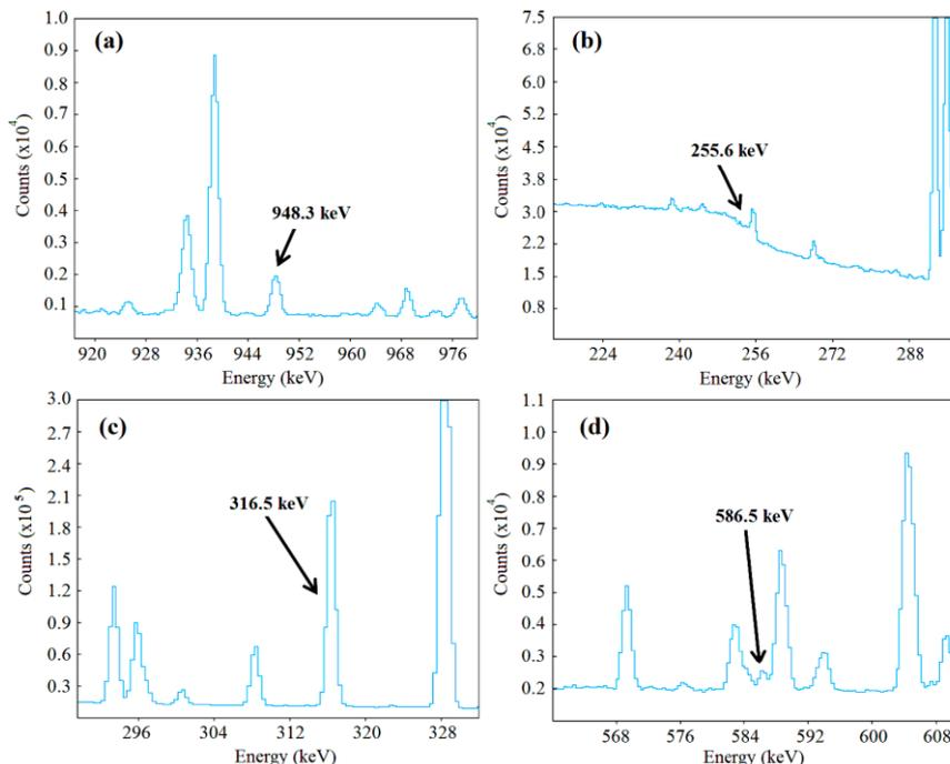
**Fig. 4.** Characteristic  $\gamma$ -rays in the spectra taken after the end of the irradiation which correspond to the (a) Au(n,4n), (b) Au(n,5n), (c) Au(n,6n) and (d) Au(n,7n) channels, respectively.
