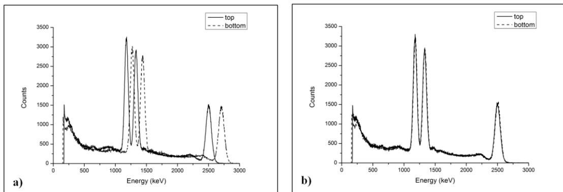
**Fig. 4.** a) Spectrum from the top and bottom segment of the crystal before the adjustment and b) after the adjustment.
