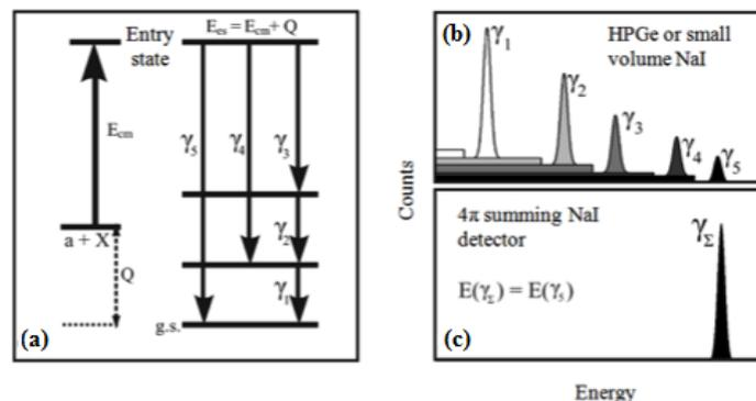
**Fig. 1.** Typical spectra (b) from HPGe or small volume NaI detector and (c) from a large-volume  $4\pi$  summing NaI detector for the de-excitation of a compound nucleus (a) [1].
