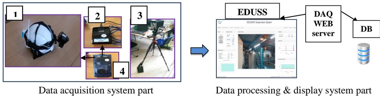
**Fig. 4.** DAQ System sources: (1) Mobile Personal Supervision System (MPSS) (2) Sensor Board (PTU) (3) Gamma radiation camera (4) Dosimeter for radiation data. The right part of the figure presents the data processing and display of the system part.
