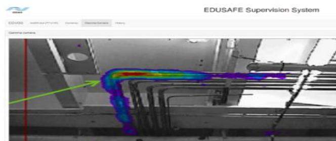
**Fig. 3.** Gamma camera image displayed in EDUSS GUI.
