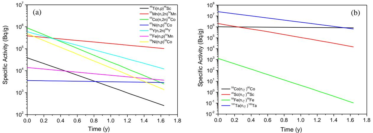
**Fig. 3.** Specific activity with time after the end of irradiation for the radionuclides produced by (a) threshold and (b) neutron capture reactions in the dosimetry foils
