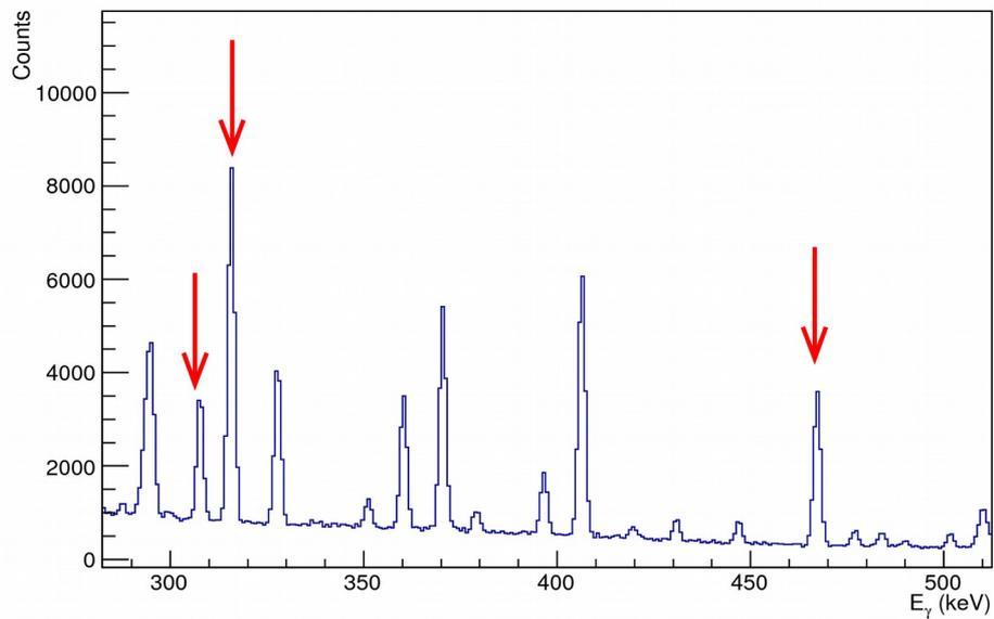
**Fig. 3.** Part of the  $\gamma$ -ray spectrum of the Iridium sample as resulted after the 10 MeV irradiation. The  $\gamma$ -ray lines (308 keV, 316 keV and 468 keV) that were used in the analysis are indicated with red arrows.
