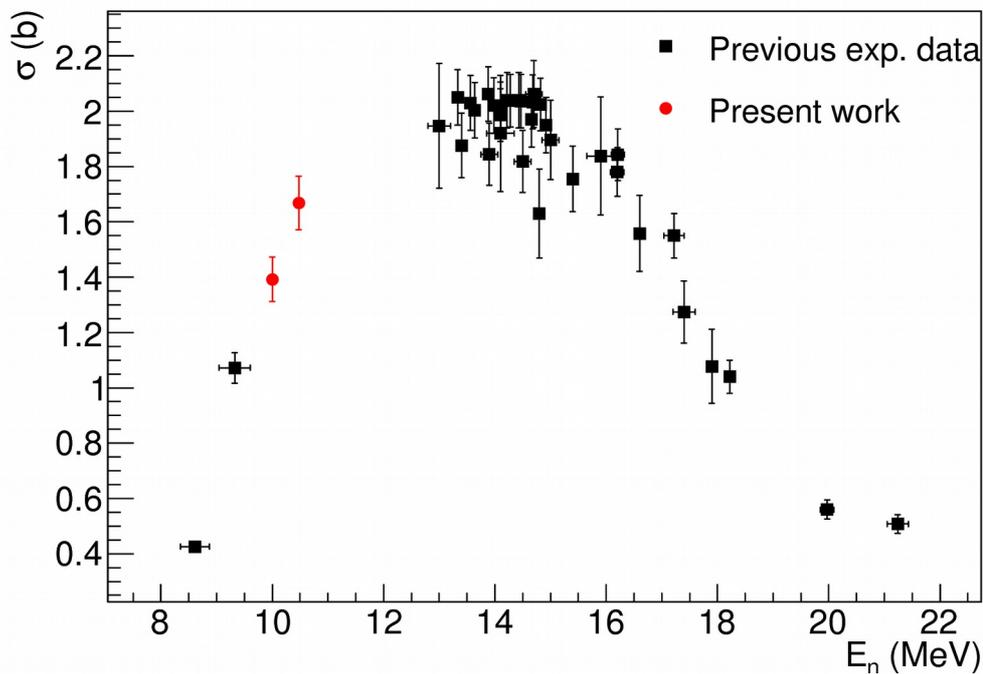
**Fig. 4.** Available experimental cross section data for the  $^{193}\text{Ir}(n,2n)^{192}\text{Ir}$  reaction according to the EXFOR data base [2] along with the cross section data resulted from the present work (red bullets) .
