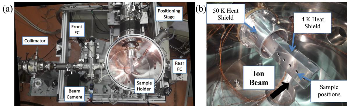
**Fig 1.** (a) Top view of the upgraded system commissioned at the accelerator lab; (b) sample holder attached to the new 4K cold-head.
