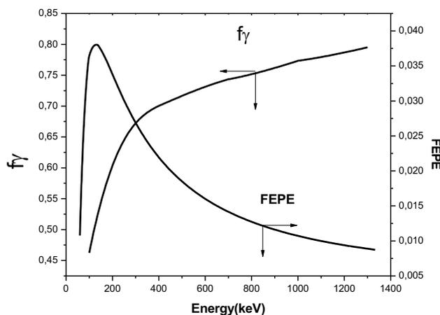
**Fig. 2** FEPE for point source and MCNP derived large sample to point efficiency transfer factor ( $f_\gamma$ ) as a function of photon energy for the counting geometry
