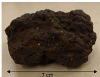
**Fig. 1** Metallurgical slag sample
