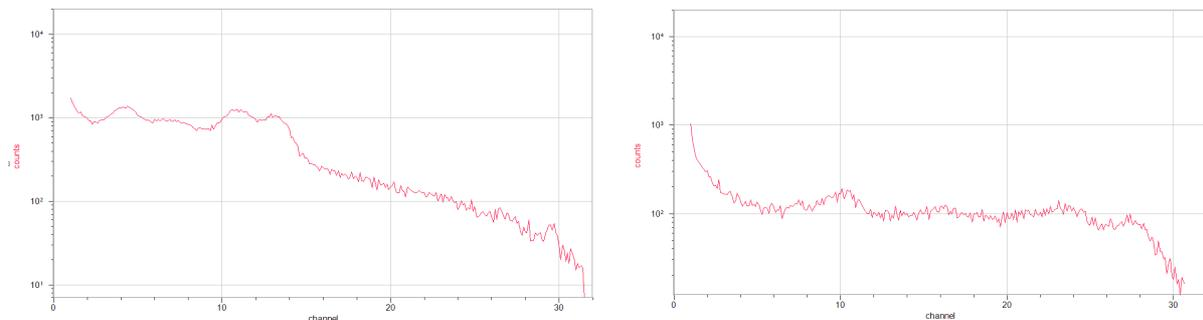
**Figure 2.** A <sup>137</sup>Cs/<sup>60</sup>Co source close to the NaI detector (left) and away from it (right) (Δt=15 min)
