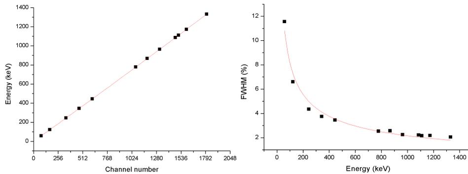
**Fig. 4** Energy calibration (left) and resolution calibration (right) of the LaBr<sub>3</sub>(Ce) scintillator
