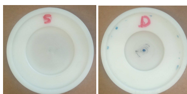
Fig. 2 The acetal holder: the source side (left) and the detector side (right)
