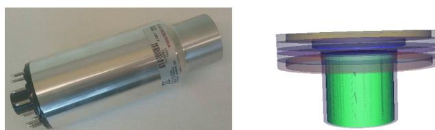
**Fig. 1** The LaBr<sub>3</sub>(Ce) detector (left) and MCNPX simulation of the gamma area source (right)
