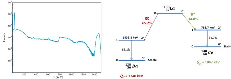
**Fig. 3** Background spectra of LaBr<sub>3</sub>(Ce): Internal activity of <sup>138</sup>La (T<sub>1/2</sub> = 1011 y) and <sup>227</sup>Ac (T<sub>1/2</sub> = 21.77 y) in the energy range 0 – 1500 keV (acquisition time 54000 sec) and <sup>138</sup>La decay diagram
