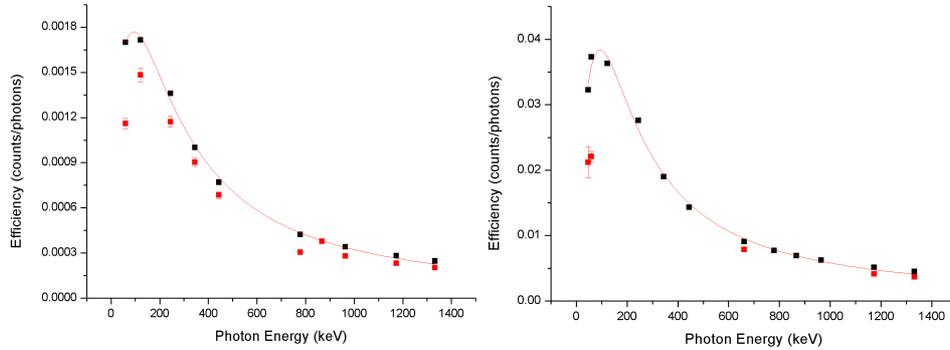
**Fig. 5** Efficiency calibration curves for the geometries (PS) (left) and (VS) (right) with the corresponding selected fitting functions for the MCNPX data:  $y = (2.874 x^{0.394}) / (7444 + x^{1.703})$ ,  $R^2 = 0.998$  and  $y = (38.413 x^{0.587}) / (9800 + x^{1.857})$ ,  $R^2 = 0.995$
