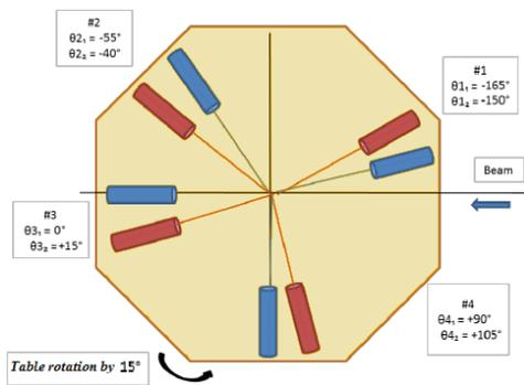
**Figure 1.** A sketch of the experimental setup
