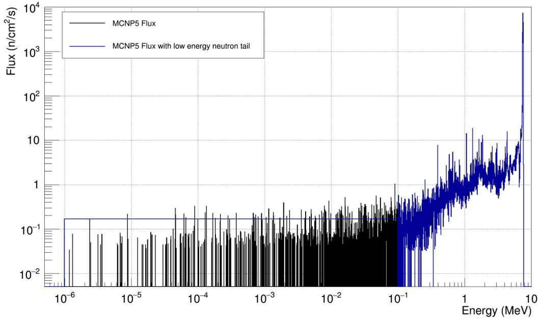
**Fig. 4.** MCNP5 flux results and the low energy neutron flux used for the estimation of the parasitic neutrons at 7.5 MeV energy of the main neutron beam
