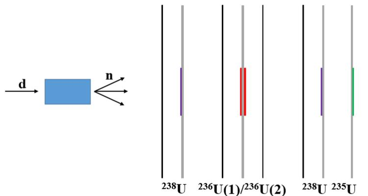
**Fig. 2.** Schematic view of the Micromegas detectors (black) and targets (grey) assembly
