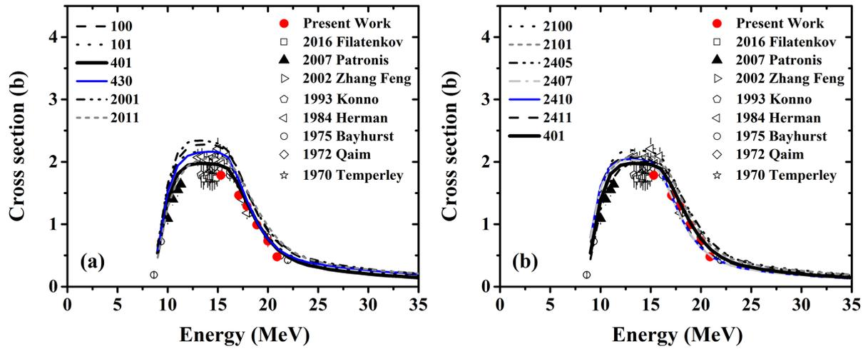
**Fig. 2:** Experimental results of the present work along with existing data in literature [10] and theoretical calculations results with EMPIRE 3.2.2 [4,5] for the  $^{191}\text{Ir}(n,2n)^{190}\text{Ir}^{g+m1+0.086m2}$  reaction and for every optical model potential presented in Table 1.
