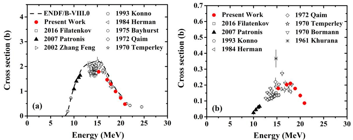
**Fig. 1:** Experimental results of the present work for the (a)  ${}^{191}\text{Ir}(n, 2n){}^{190}\text{Ir}^{g+m1+0.086m2}$  and (b)  ${}^{191}\text{Ir}(n, 2n){}^{190}\text{Ir}^{m2}$  reaction channels, along with previously existing data in literature [10] and ENDF/B-VIII.0 [11] evaluation (dashed curve), when is available.
