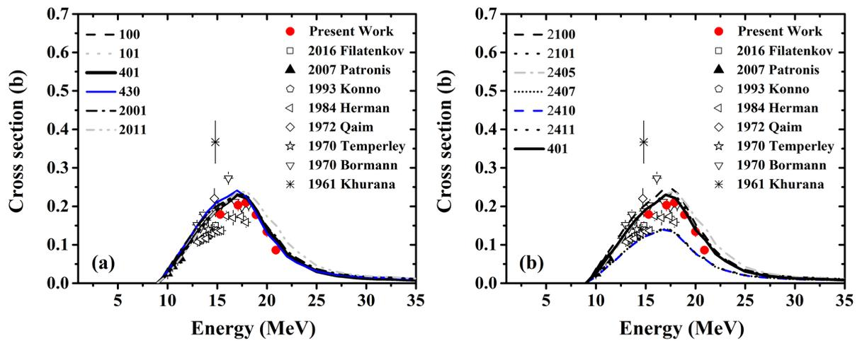
**Fig. 3:** Experimental results of the present work along with existing data in literature [10] and theoretical calculations results with EMPIRE 3.2.2 [4,5] for the  $^{191}\text{Ir}(n,2n)^{190}\text{Ir}^{m2}$  reaction and for every optical model potential presented in Table 1.
