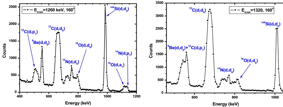
**Fig. 1.** (a) and (b) Experimental d-EBS spectrum at  $E_{d,lab} = 1260$  keV,  $\theta = 160^\circ$  and  $E_{d,lab} = 1320$  keV,  $\theta = 160^\circ$ , respectively along with the corresponding peak identification
