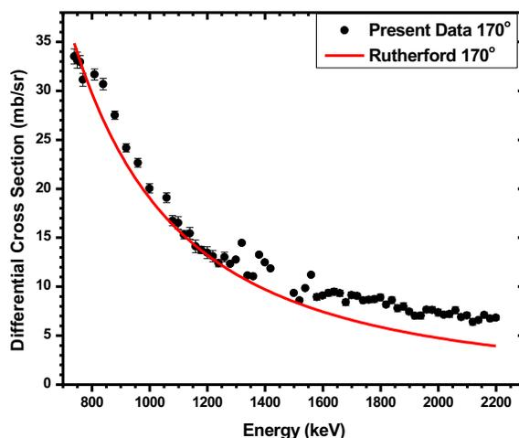
**Fig. 4.** (a)-(e) Differential cross section values (mb/sr) of the  ${}^9\text{Be}(d,d){}_9\text{Be}$  elastic scattering measured at  $E_{d,\text{lab}} \sim 740\text{-}2200$  keV and for the scattering angles of  $120^\circ$ ,  $140^\circ$ ,  $150^\circ$ ,  $160^\circ$ , and  $170^\circ$ , in variable steps, along with data from literature. The total statistical uncertainties are included in the graphs; the uncertainties are not visible in the horizontal axis due to the selected scale
