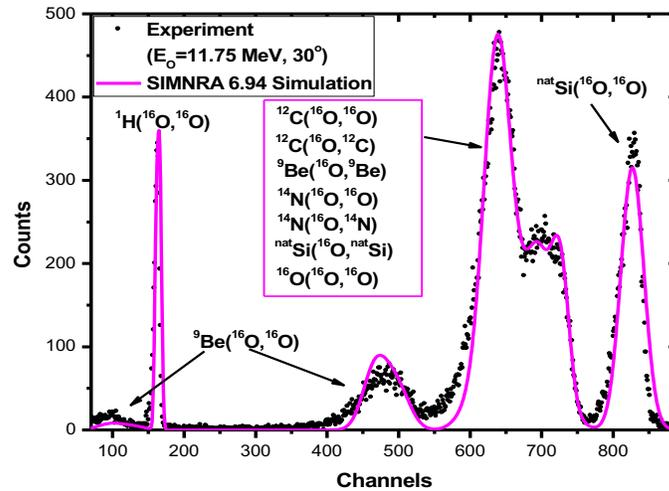
**Fig. 3.** Experimental and SIMNRA simulated, transmission ERDA spectrum at  $E_{o,\text{lab}}=11.75 \text{ MeV}$  and the scattering angle of  $30^\circ$ , along with the corresponding peak identification.
