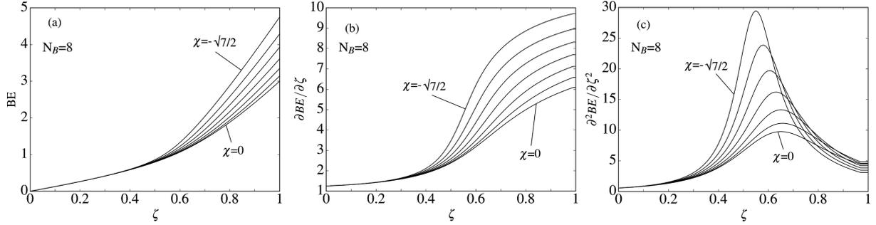
**Fig. 3.** (a) Binding energy, the (b) first and (c) second derivatives over  $\zeta$  and for various  $\chi$  parameters. The CP of the QSPT is defined by the location of the maximum in the second derivative.
