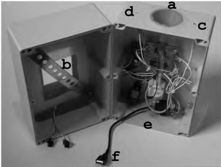
**Figure 2.** Representation of the external interface. (a) Funnel or water drainage (b) Window for the iPaq display with holders, (c) light sensor, (d) temperature sensor, (e) exit of the water, (f) iPaq's cradle connector
