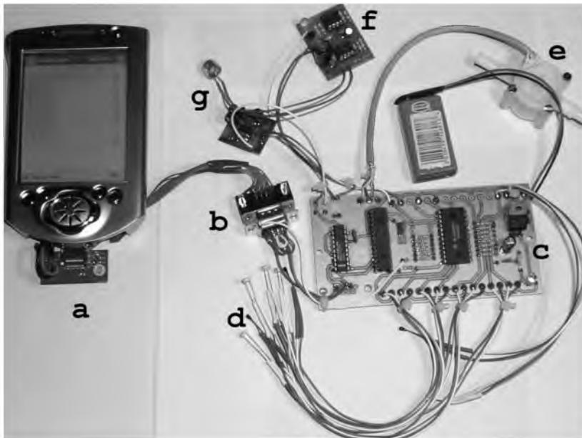
**Figure 1.** Sensors interfacing with the iPaq. (a) iPaq pocket pc and the cradle, (b) serial connection with the sensor board, (c) interfacing board, (d) temperature and light sensors (a pair for each side of the box excluding the bottom), (e) flow sensor to detect 'watering', (f) clap sensor, (g) three-axes accelerometer (We incorporated a clap sensor and an accelerometer for further interactions improvements of the interface)
