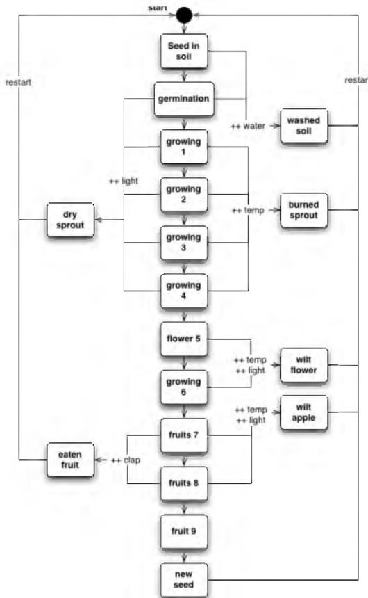
**Figure 4.** Software state chart. To proceed through the main flow of interaction the child should provide the right amount of water, and light and temperature exposure of the box. Over- or under-providing the right conditions brings the simulation to one of the unhealthy states on the sides. Prolonged mistreatment of the box kills the simulated plant and the cycle is restarted
