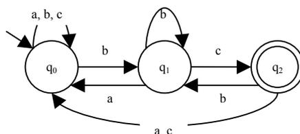
**Figure 1:** Local non-determinism in an almost deterministic automation
