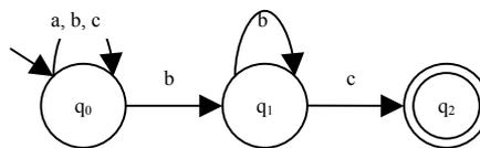
**Figure 2:** Redundant transitions in a non-deterministic automation
