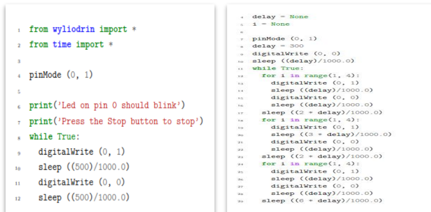
Figure 6. Python code for LED blink and Buzzer SOS applications
