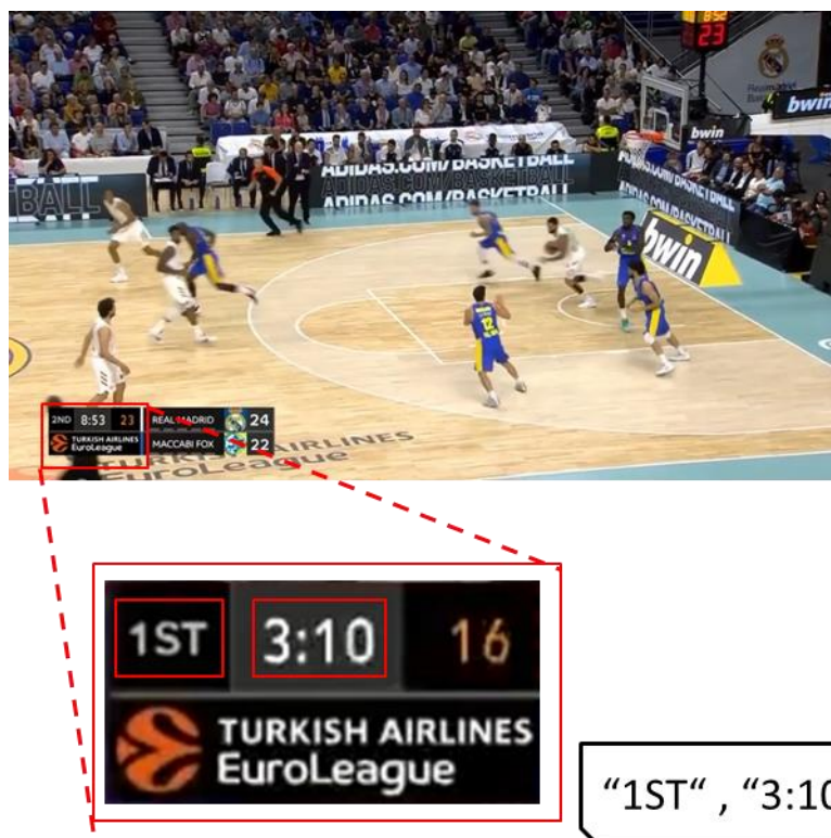
Figure 6: Detection, recognition, and extraction of the match clock to align the textual events with the timelines of the video segments (Anagnostou, 2022).
