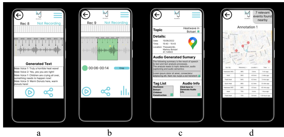
Figure 3: (a) Once dictation is finished the application provides the generated text, (b) option to extract a specific part of the recorded audio, (c) identified topic and information regarding the captured audio along with auto-generated summary and tag list, (d) relevant (by topic) nearby events
