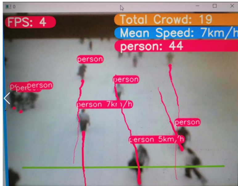
Figure 9: Processing of images in real time
