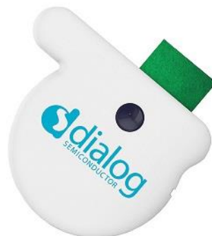
Image 1. Dialog Semiconductor 14583 IoT Sensor Board (source: https://www.digikey.sg/en/products/detail/dialog-semiconductor-gmbh/DA14583IOTSENSDNGL/5887065 )
